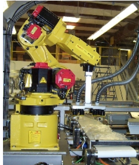
Sabel Engineering's TL-10 robotic, top-load, case packer uses three conveyors to index bags of Mamacita's empanada dough, simultaneously build cases, and pack 90 bags/min. with less errors, wiring, and repetitive motion.
